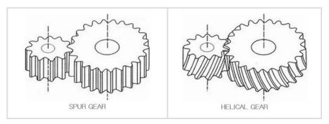
Fig. 1 Two sets of gears. Individual spur gears have a wider class of exact symmetries than individual helical gears, but the latter can have approximately the same symmetries for sufficiently small helix angles. Image by Ningbo Twirl Motor Co., Ltd.: http://www.twirlmotor.com/Blog/Industry-news/new-12.html
